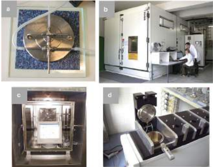
Fig. 2 Different devices for emission testing of building products. (a) FLEC; (b) 48 m 3 stainless-steel chamber; (c) 1 m 3 stainless-steel chamber; (d) micro chamber ( \mu -CTE)
